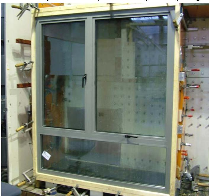
achieving a category 3 classification". The system is now part of the BM Trada quality 'Q' mark scheme and also meets all the requirements of secure by design. To achieve a rating of class 4 at 600Pa on air, 1050 Pa on water and 2400 Pa wind resistance on such a large window is a huge achievement. The safety pressure alone of 3600 Pa is a very high standard to meet for any window system, and is the equivalent to 166 mph winds.
